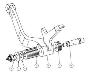
4. Tighten locknut on AK1156 (5) until the arm and wheel assembly stays up under its own weight. For installation purposes there should initially be a gap between the tire and disk. If necessary move some adjusting washers from outside of the arm to inside position to create a gap. This gap will be eliminated in step 8. Occasionally it may be necessary to move the hub of the arm out onto the adjusting stud.
