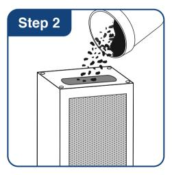
Using a cup or funnel, carefully pour activated carbon into filter.
