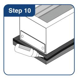
Glue joins of seal together by gently prying two edges apart.
