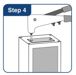
Pop rivet aluminium cap over the activated carbon.
