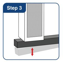
Tap the filter firmly with rubber mallet at base of filter to ensure the carbon is tightly packed. Continue to top up as carbon settles.
