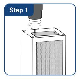
Remove all dust pads. Drill out pop rivets on both end caps and remove the carbon and indicator beads inside. Using compressed air, remove dust and dirt from the filter.
