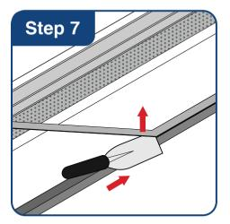
Remove old foam seals from filter, taking note of where seals are placed as some filters will have multiple seals of different sizes. Remove any residual adhesive from the filter.
