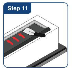
Replace foam dust pads with a small paint scraper, ensuring the pink/white media is closest to the carbon bed with the pink side facing down.
