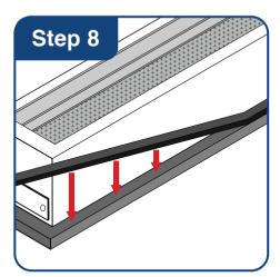
Apply new seals to the correct position on the filter.
