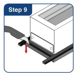
Cut the corners of the seal with a sharp blade to create right angles.
