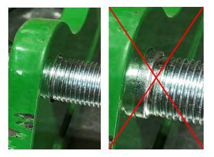
2. Install the bolts through the row unit/support plate holes then through the flange bushings in the parallel arms.
