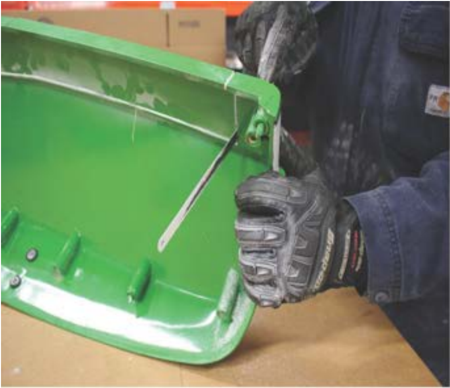
Next cut the remaining corners with hacksaw blade.
