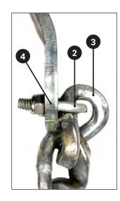
Using one u-bolt 2 on each side, attach drag chain 3 to chain bracket 4. Secure with nuts. Using 7/16" socket, tighten u-bolts on chain.
