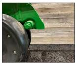
Release spring  $oldsymbol{1}$  to remove tension from closing system.
