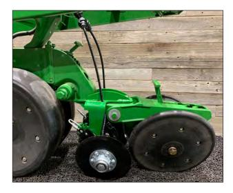
Install orifice plates  $oldsymbol{0}$  in the rubber grommets  $oldsymbol{20}$ .
